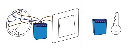
• **FITTING:** Mini Dimmer fits **all types of flush mounting boxes worldwide**. Reduce assembly time and installation expenses. Install it fast and easy behind a classic switch.
