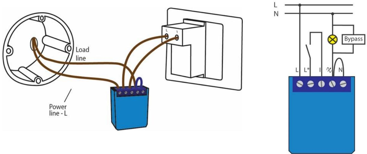
① NOTE: When installing the Mini Dimmer in a 2-wire installation we recommend using a Bypass.
