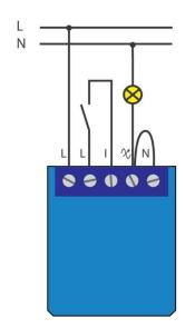
2-wire installation (110 – 240 Vac) With Bypass
