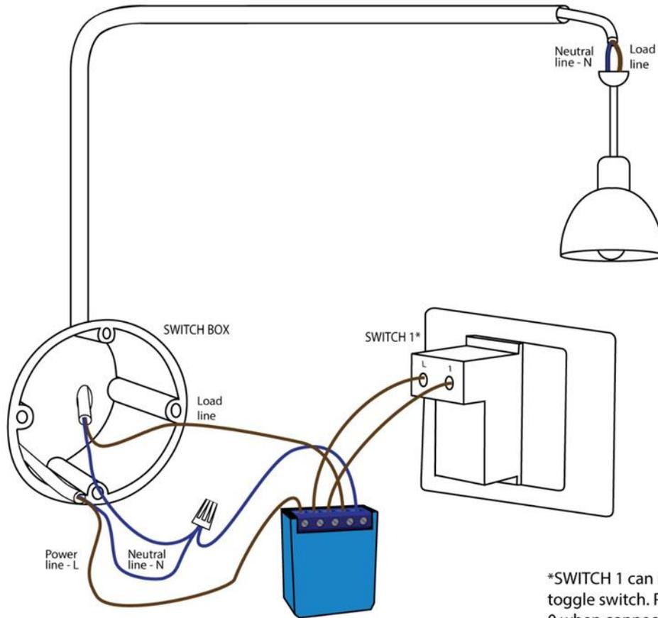
\*SWITCH 1 can be a momentary switch or a toggle switch. Please set parameter 1 to value 0 when connecting to a momentary switch (default setting). Set parameter 1 to value 1 when connecting to an on/off toggle switch. Please see the Configuration Parameters chapter for more information about advanced parameter settings
